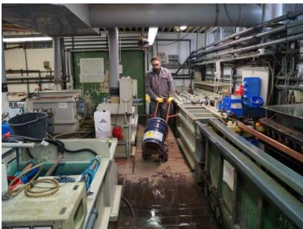
Photograph shows worker transferring a drum containing chromium trioxide.
