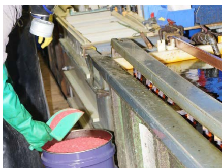
This photo shows adjustment of bath with chromium trioxide.
