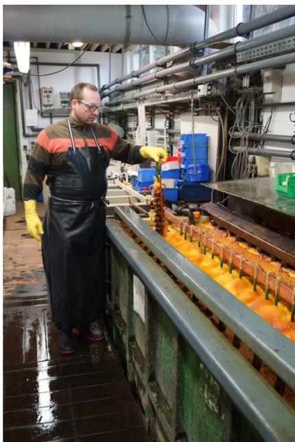
**!** Photograph shows plating at open tanks with manual loading not in compliance with this GPS as P3 filter missing.
