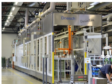
Photographs show chambers enclosing plating systems and hoist lines.
